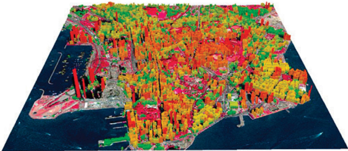
Figure 1. WUDAPT Level 2 product (3D morphological data of Kowloon Peninsula, Hong Kong) (Source: WUDAPT, 2017:7, http://www.wudapt.org/wp-content/uploads/2017/06/WUDAPT-Briefing-Doc_20170630.pdf )
